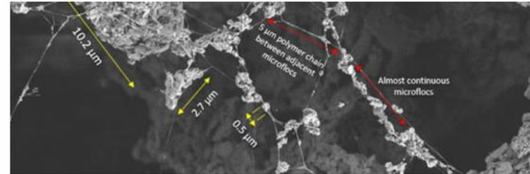
**Microstructure of kaolinite floc as revealed by cryo-SEM** - Sharma, S., Lin, C. L., & Miller, J. D. (2017). Multi-scale features including water content of polymer induced kaolinite floc structures. *Minerals Engineering*, 101, 20-29.
