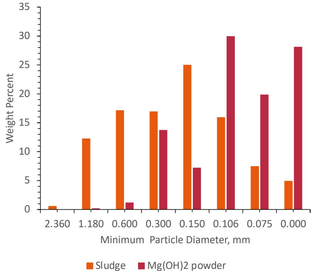
Figure 2: distribution of particle size for dehydrated sludge and magnesium hydroxide powder.
