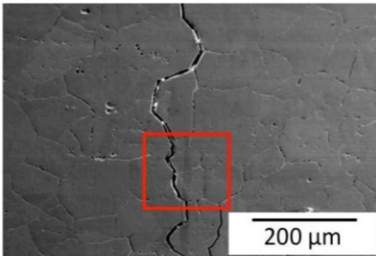
Fig. 1. Crack initiation of a stress corrosion crack [1]
