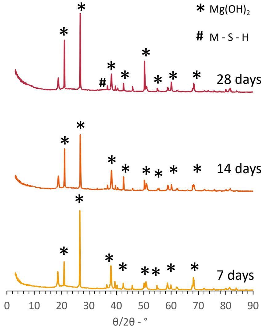
Figure 1: XRD pattern at 7, 14, 28 days for 0.375 w/s ratio cement mortar
