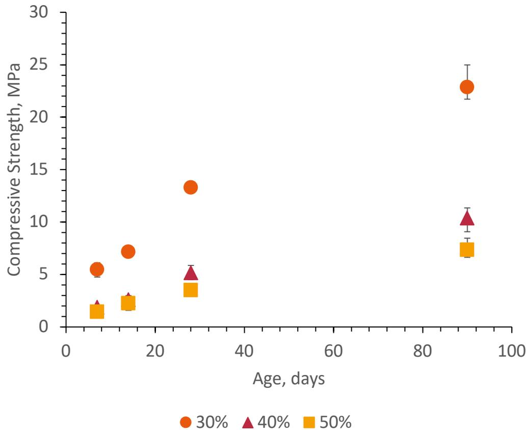
Figure 1: Compressive strength of sludge based M-S-H mortars studied for up to 90 days, for the 30%, 40% and 50% filler substitution mixes.
