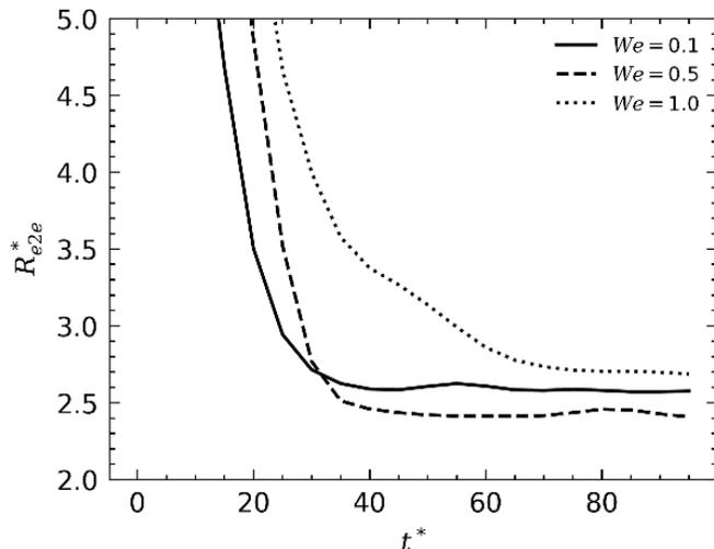
Effect of Weissenberg number,  $We$ , on temporal evolution of end-to-end polymer chain distance under shear flow conditions
