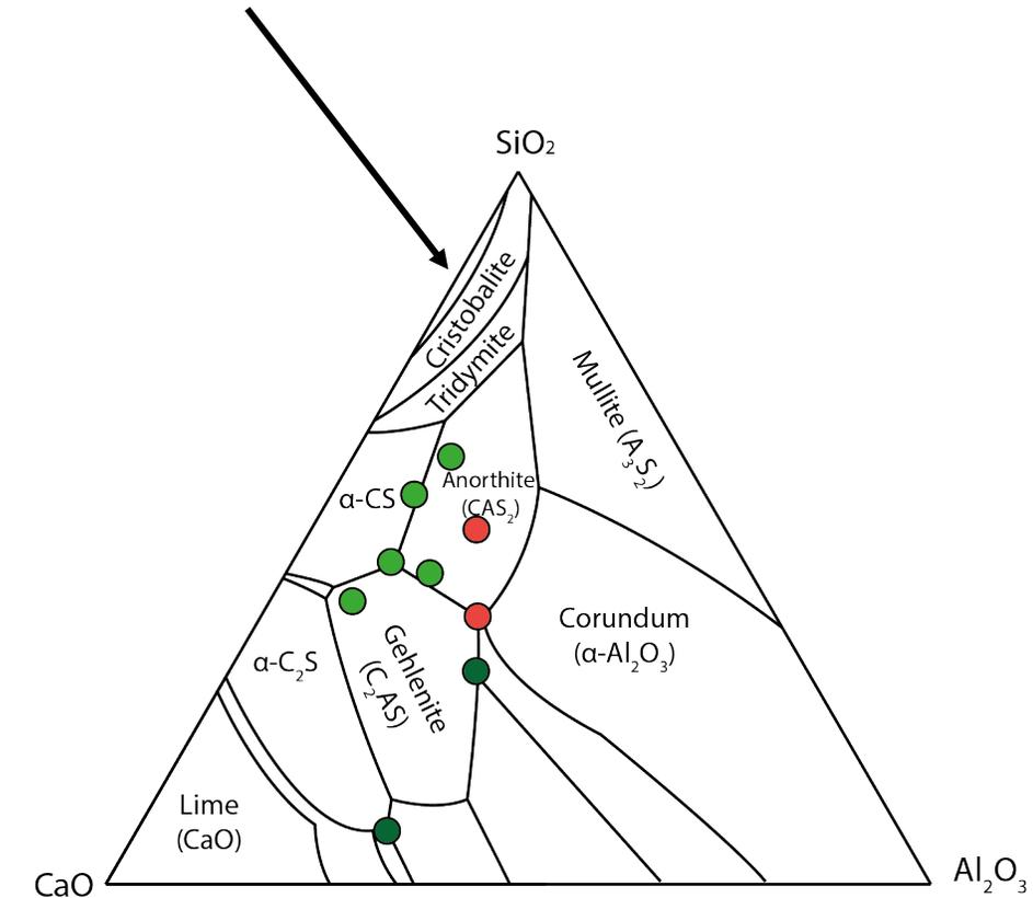
CaO, Al<sub>2</sub>O<sub>3</sub>, SiO<sub>2</sub> phase diagram with samples plotted
