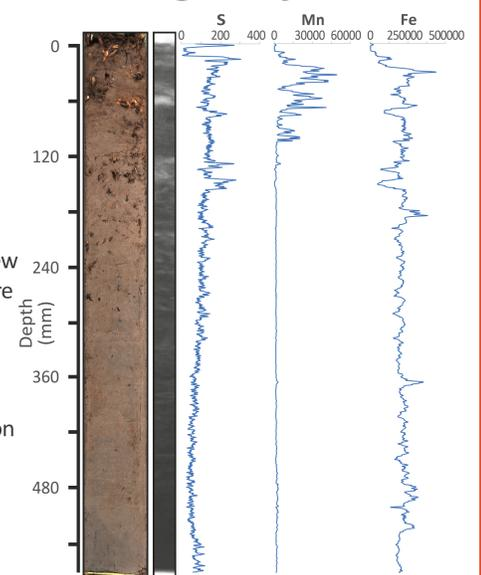
Figure 4: Optical image, radiograph and Itrax XRF scan of key stable elements in the Ravenglass sediment core before EKR treatment
