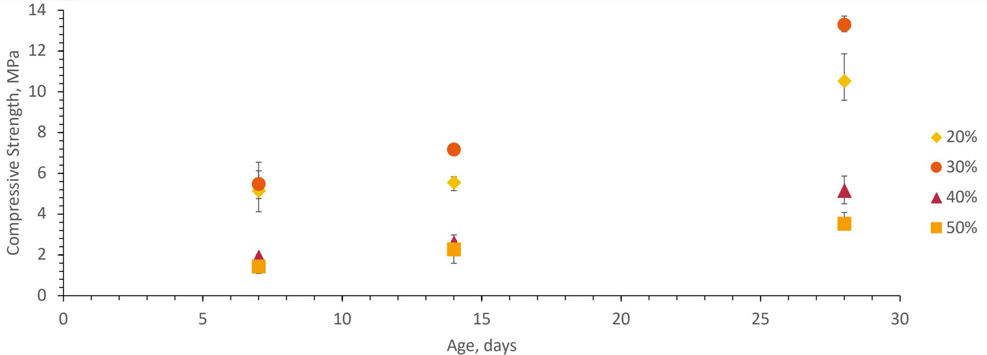
Figure 1: Compressive strength of sludge based M-S-H mortars with various proportions of silica sand filler substituted for the sludge
