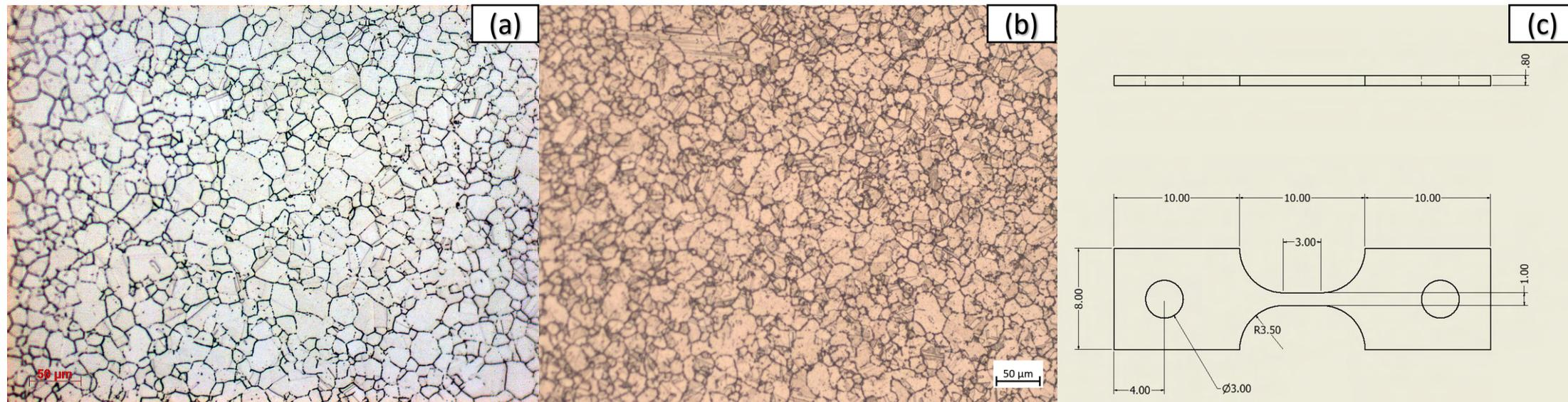
Fig. 5. Grains of etched (a) 304 stainless steel and 20/25/Nb stainless steel; (c) tensile sample design
