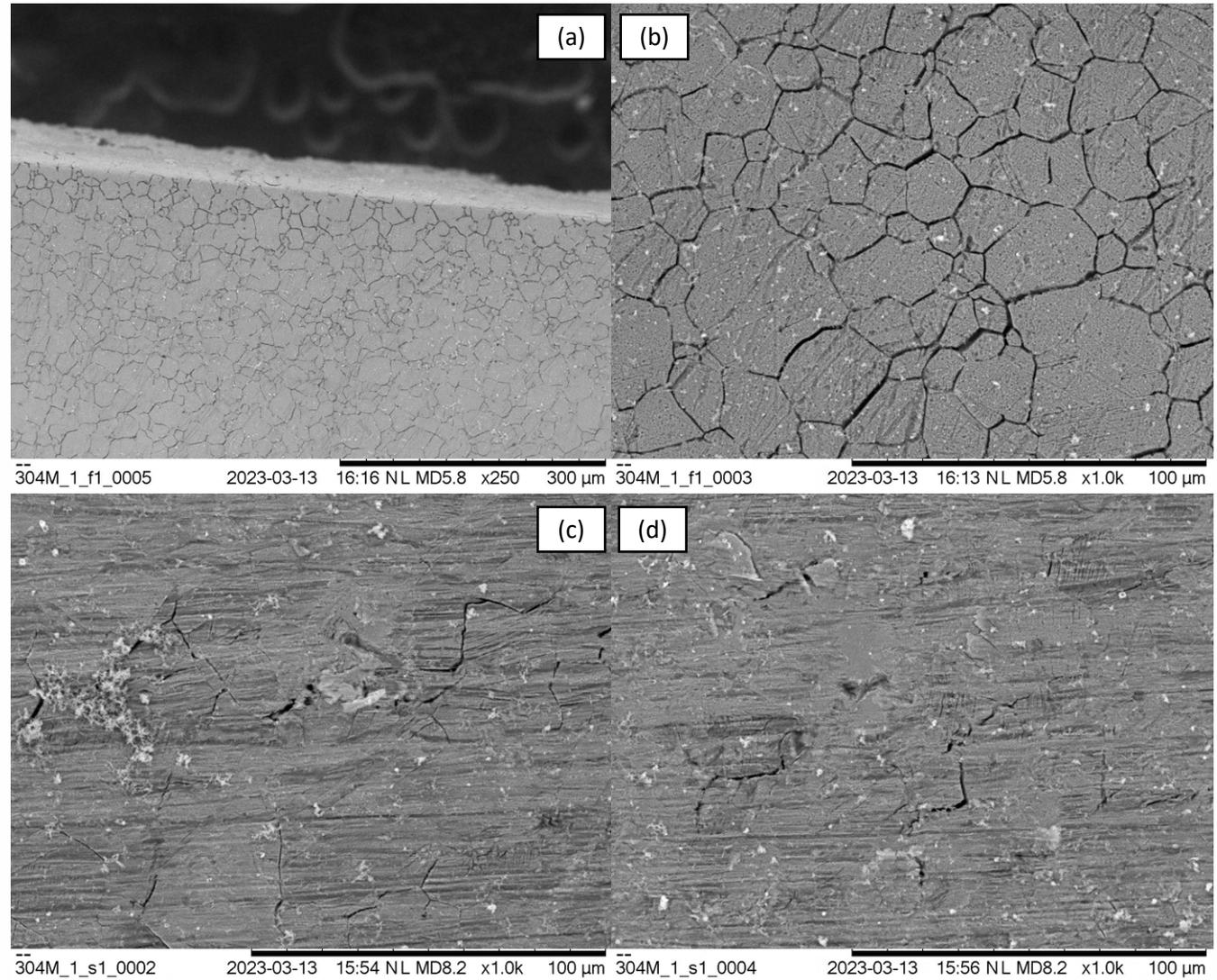
Fig. 16. SEM images of the fine surfaces of sample 2 (304 with mixed surface finish): (a), (b): face; (c),(d) edge
