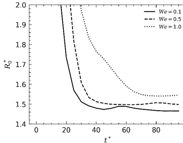
Effect of Weissenberg number,  $We$ , on temporal evolution of polymer chain radius of gyration under shear flow conditions
