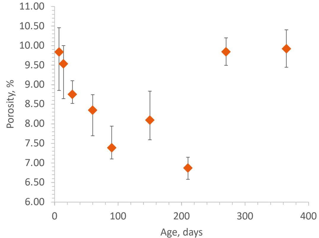
Figure 2: Porosity for the MgO based mortar at ages up to a year
