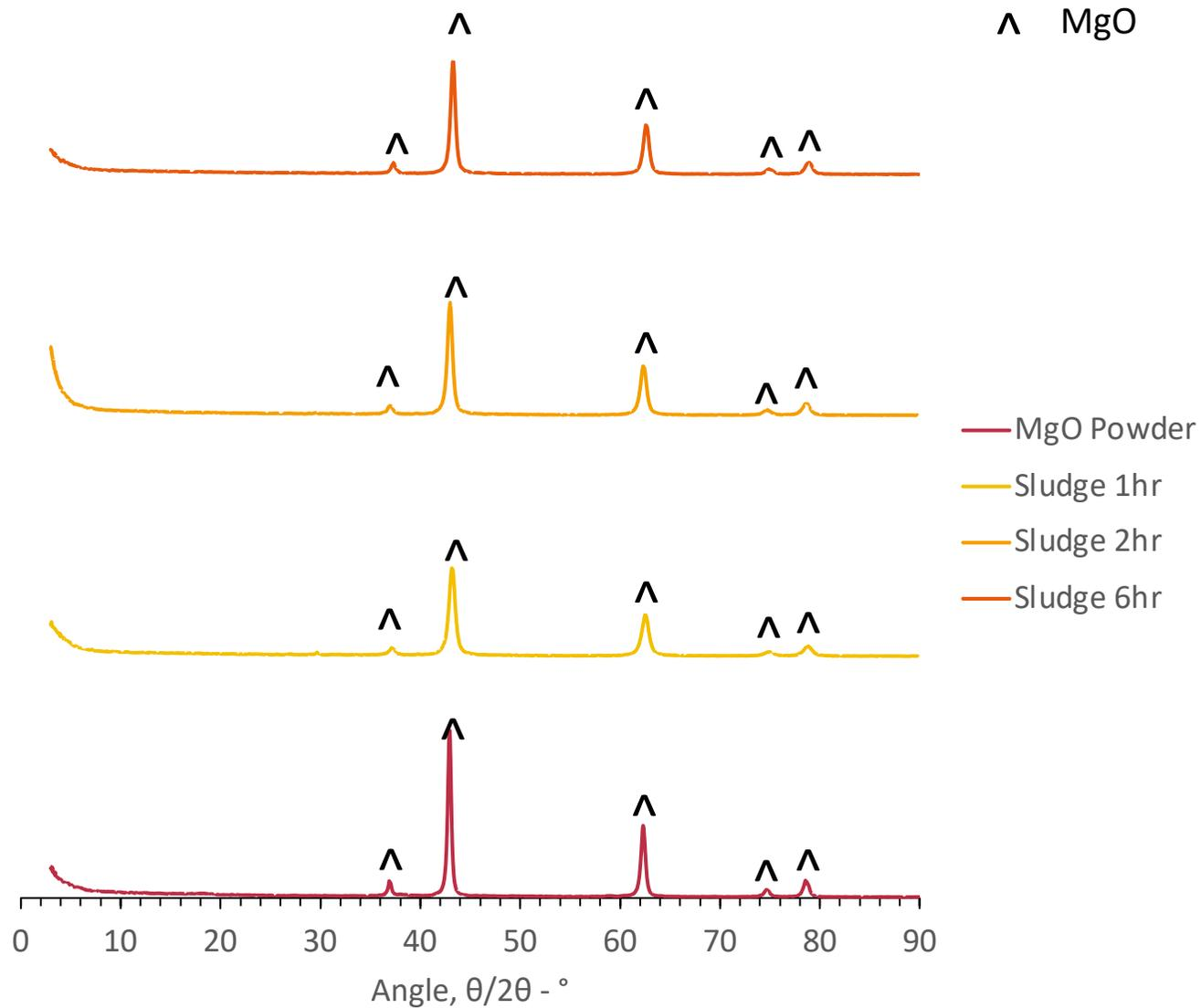
Figure 1: XRD pattern for MgO powder and brucite heated in a furnace at 600°C for various times
