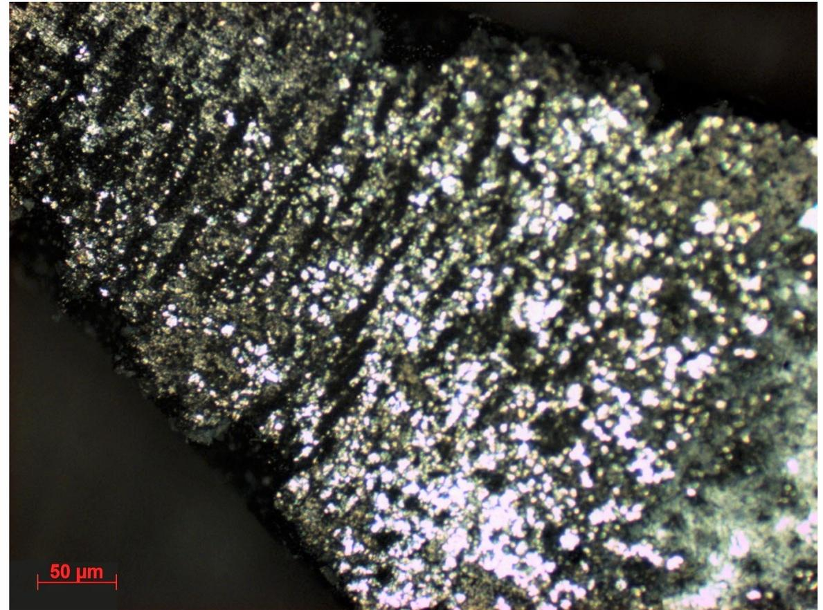
Fig. 6. Stress corrosion cracks on the surface of the a self loading tensile sample
