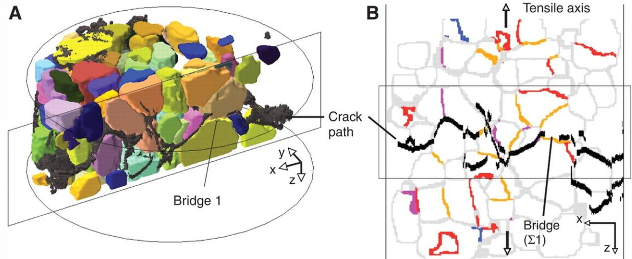
Fig. 2. DCT (diffraction contrast tomography) image showing the propagation of SCC in 3D [2]
