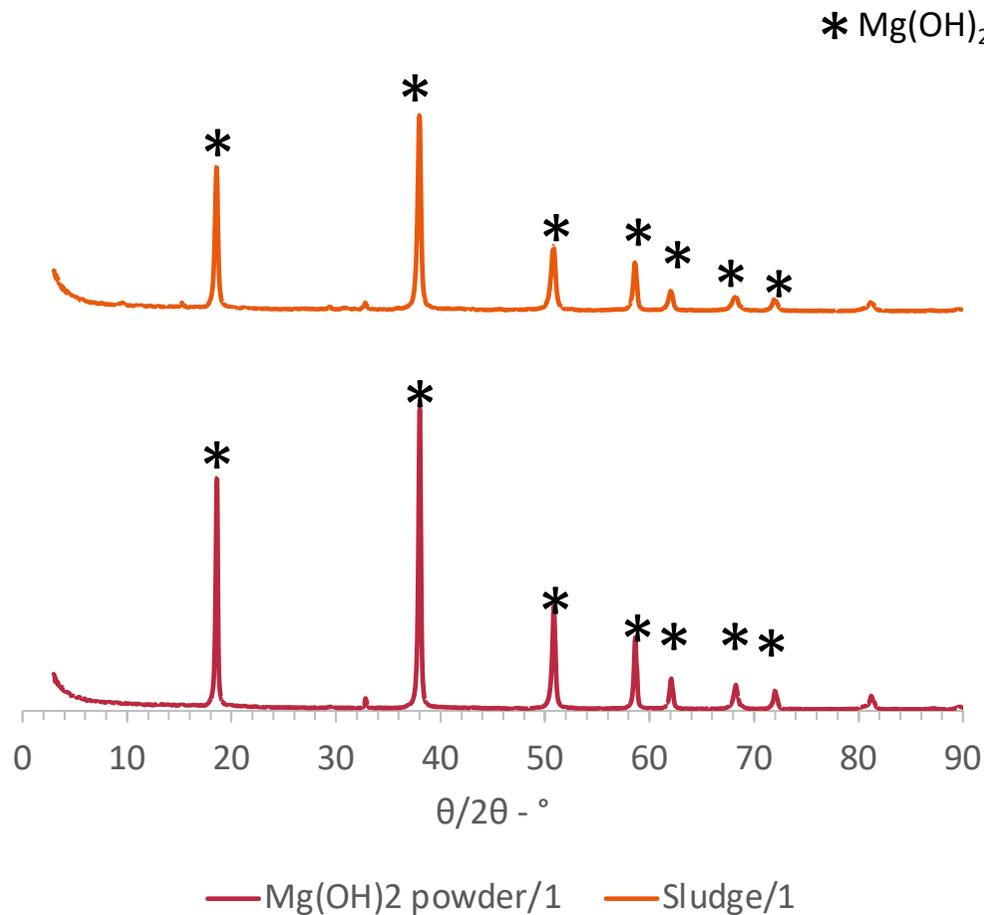
Figure 1: XRD patterns for the Mg(OH)<sub>2</sub> powder and the dehydrated sludge.
