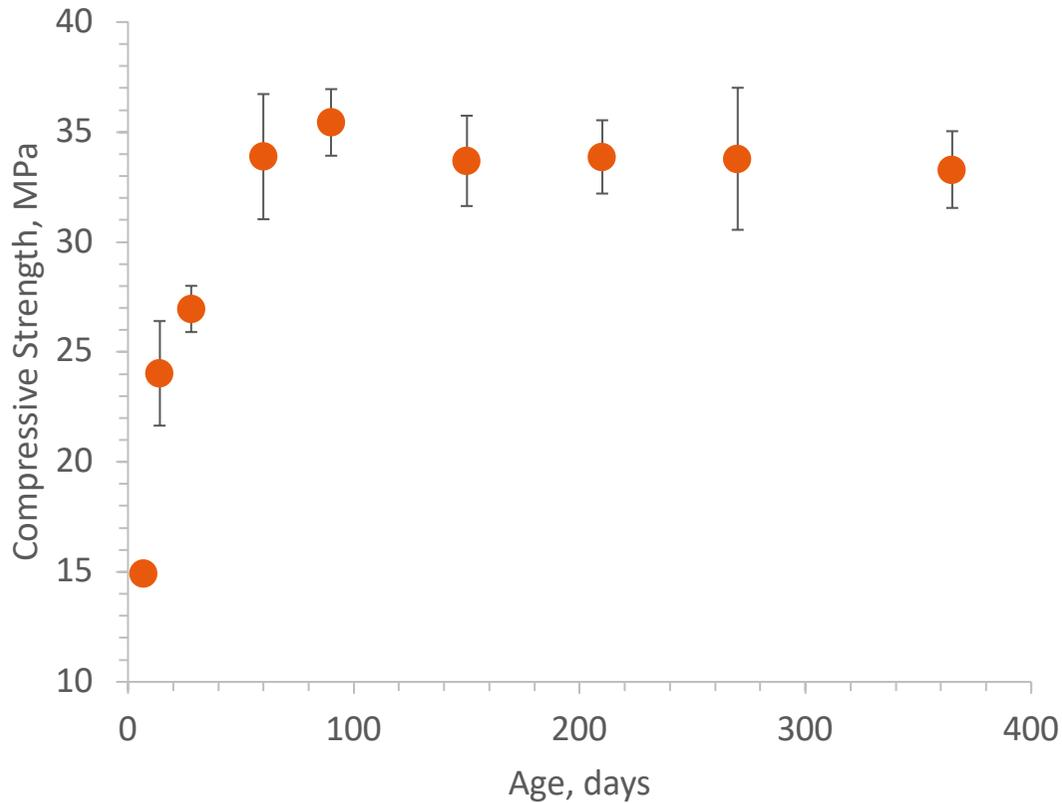
Figure 1: Compressive strength for the MgO based mortar at ages up to a year
