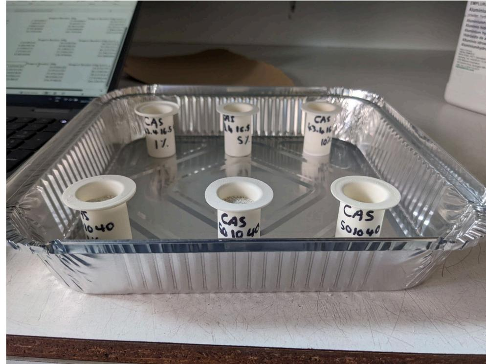
10g melt alumina crucibles to do 6 melts at a time
