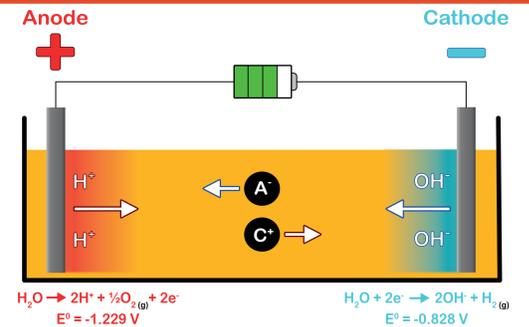
Figure 1: A typical electrokinetic cell. C<sup>+</sup> are cations and A<sup>-</sup> are anions
