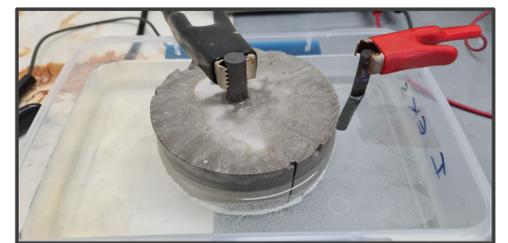
Figure 2: **Left** - trial cement core undergoing electrokinetic treatment. **Right** - schematic showing how the core was cut, and the naming convention for each section
