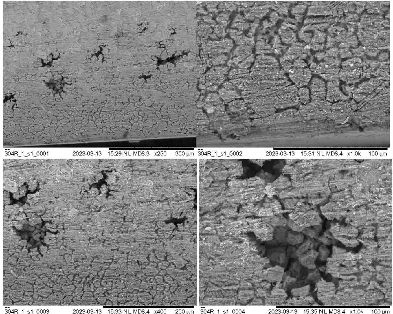
Fig. 15. SEM images of the edge of the sample 1 (rough 304 sample)
