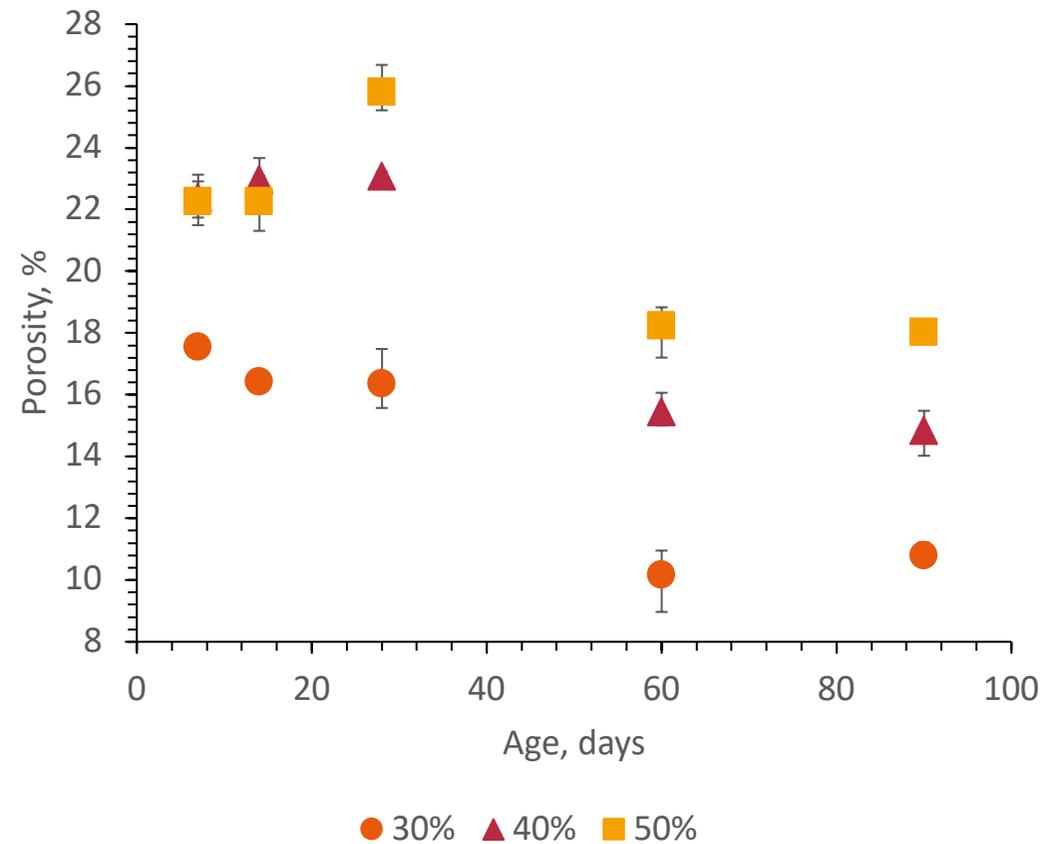
Figure 2: Porosity of sludge based M-S-H mortars studied for up to 90 days, for the 30%, 40% and 50% filler substitution mixes.
