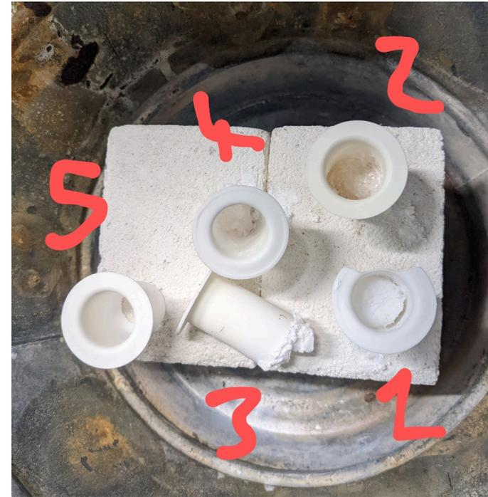
10g melt alumina crucibles most of which didn't melt
