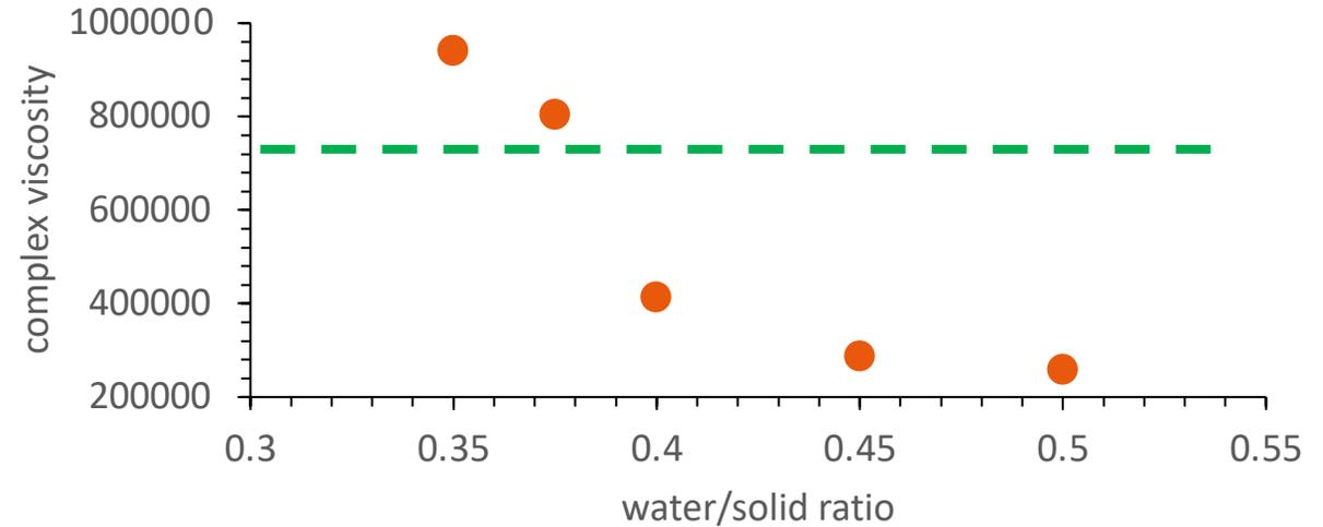
Figure 2: Decreasing viscosity with increasing water/solid ratio
