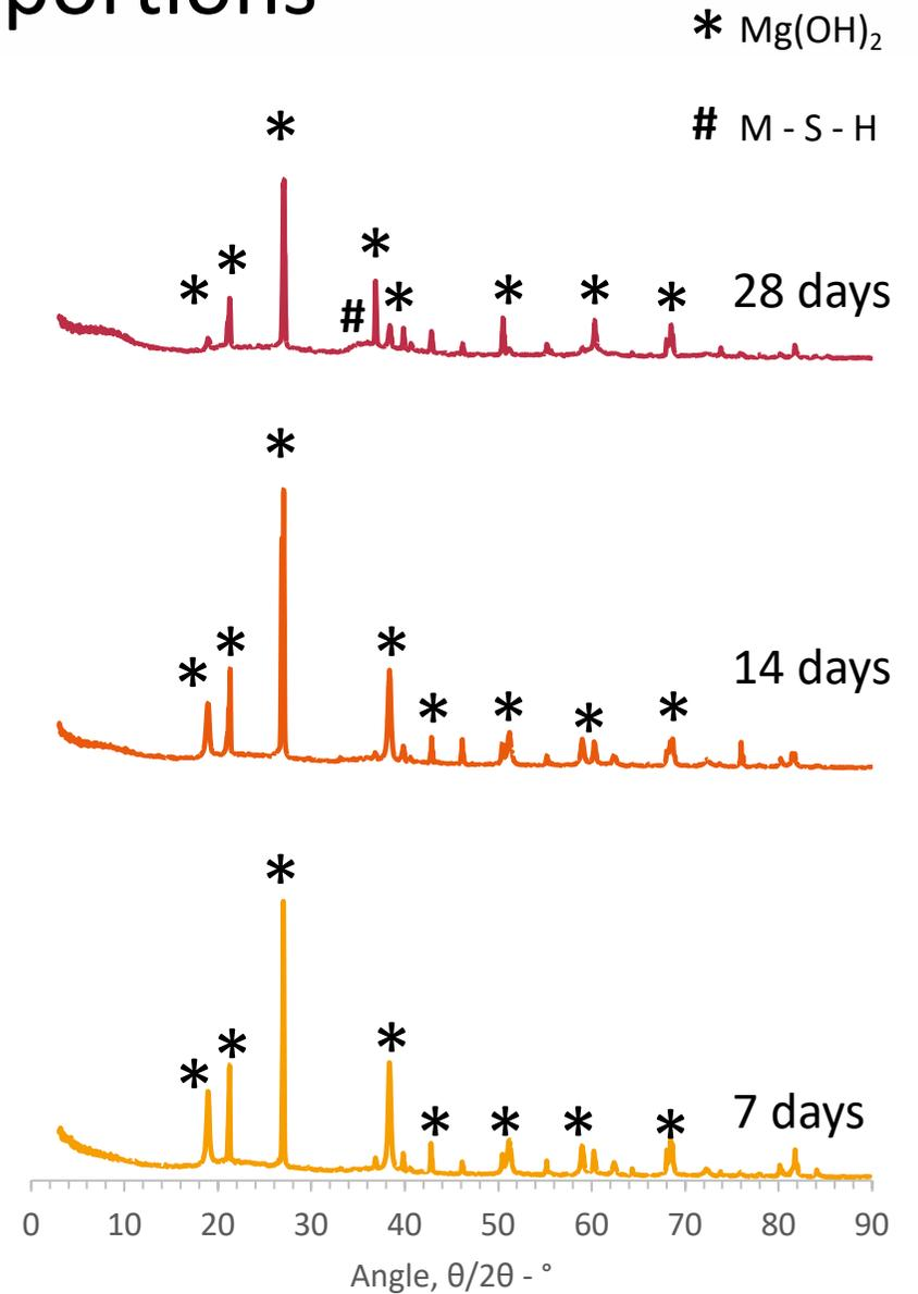
Figure 2: XRD pattern for the M-S-H mortar over 28 days
