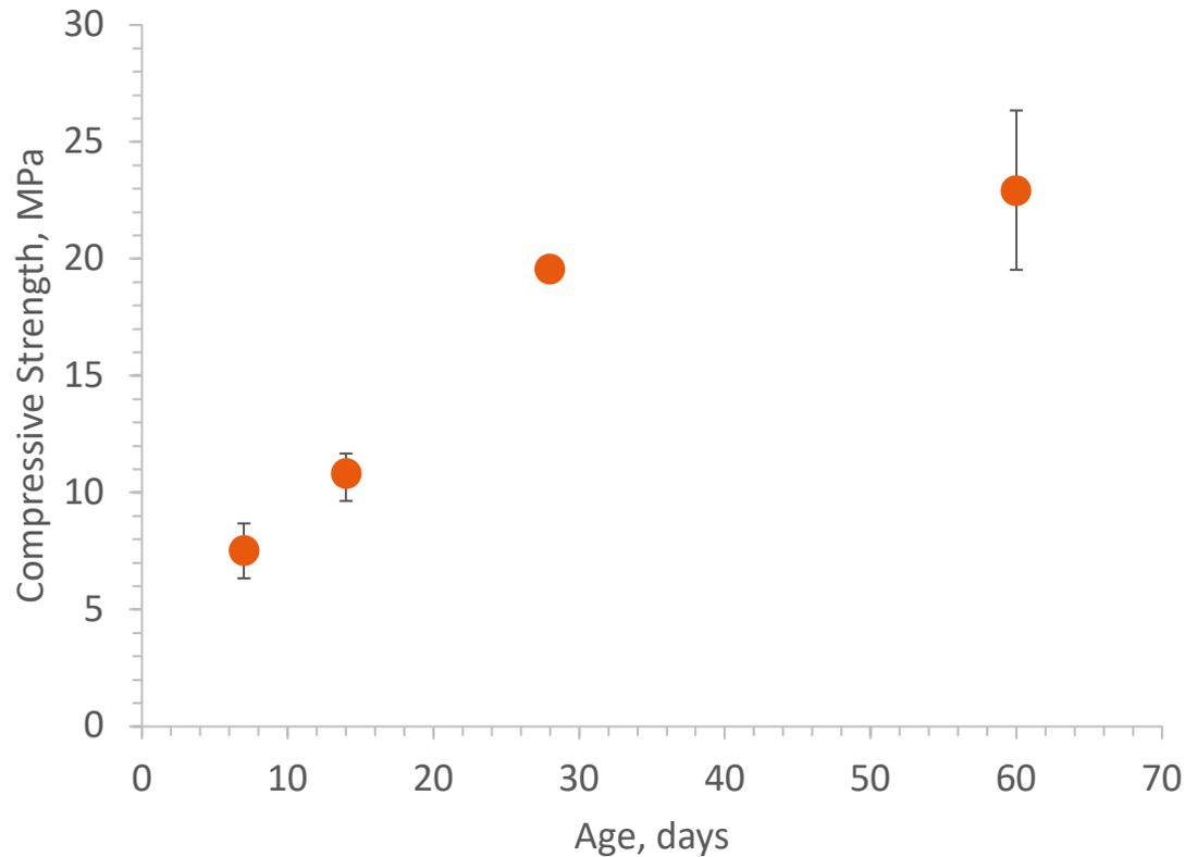
Figure 1: Compressive strength of a sludge based M-S-H mortar with sludge as the magnesium oxide component studied for up to 28 days
