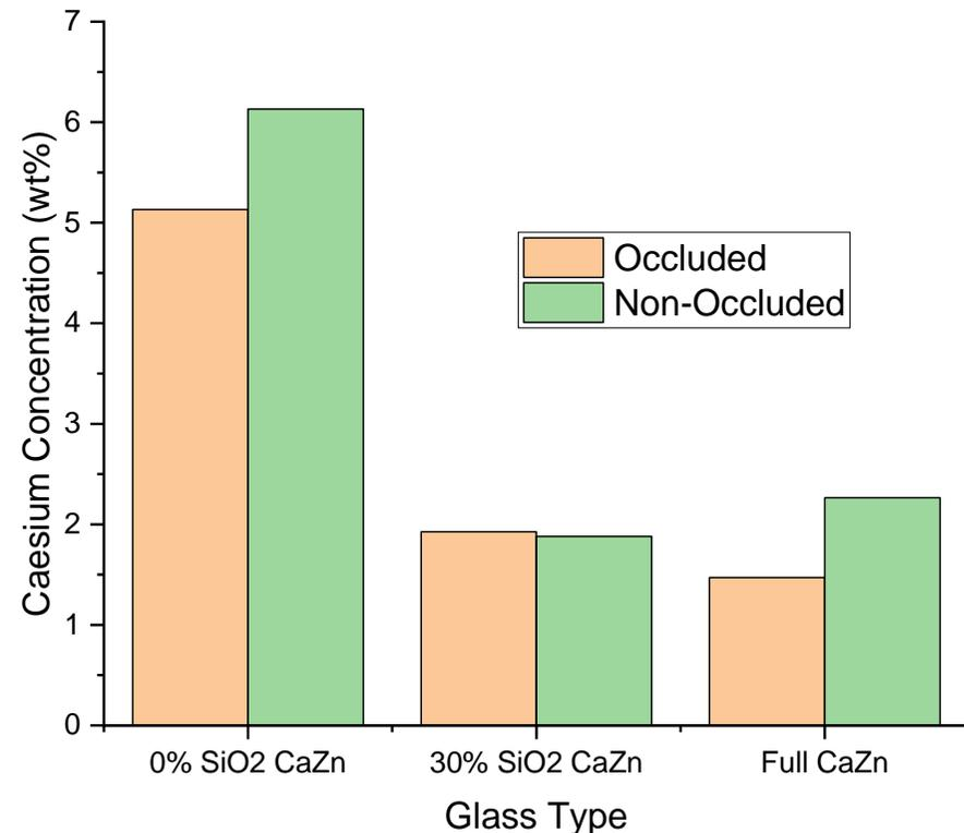
The effect of occlusion of clinoptilolite on caesium retention in three glass systems
