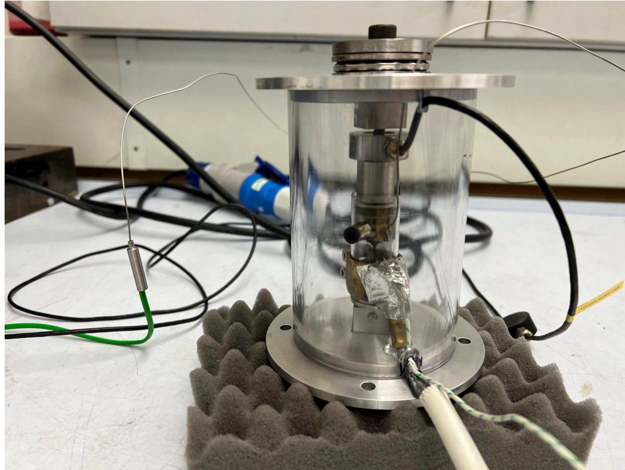
Fig. 4. Tensile rig for the in-situ synchrotron experiment
