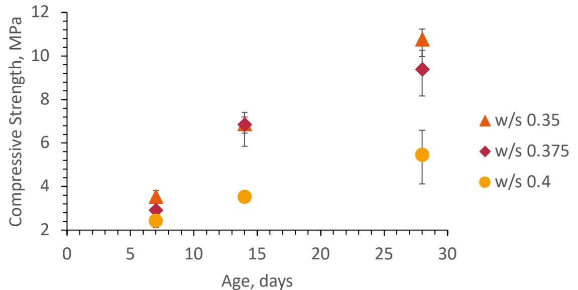
Figure 3: Decreasing strength with increasing water/solid ratio
