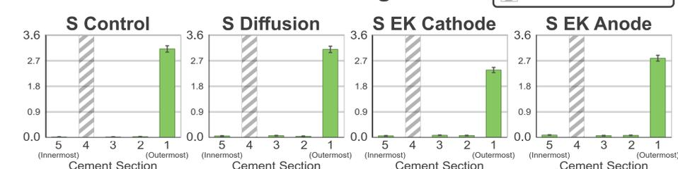
Figure 3: **Left** - <sup>137</sup>Cs data from Homogeneous-Set cores and <sup>129</sup>I data from all cores. For schematic of where each section was positioned, see figure 2 (right)
