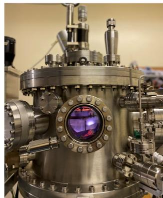
Figure 4 - Image of the sputtering kit at the University of Bristol.
