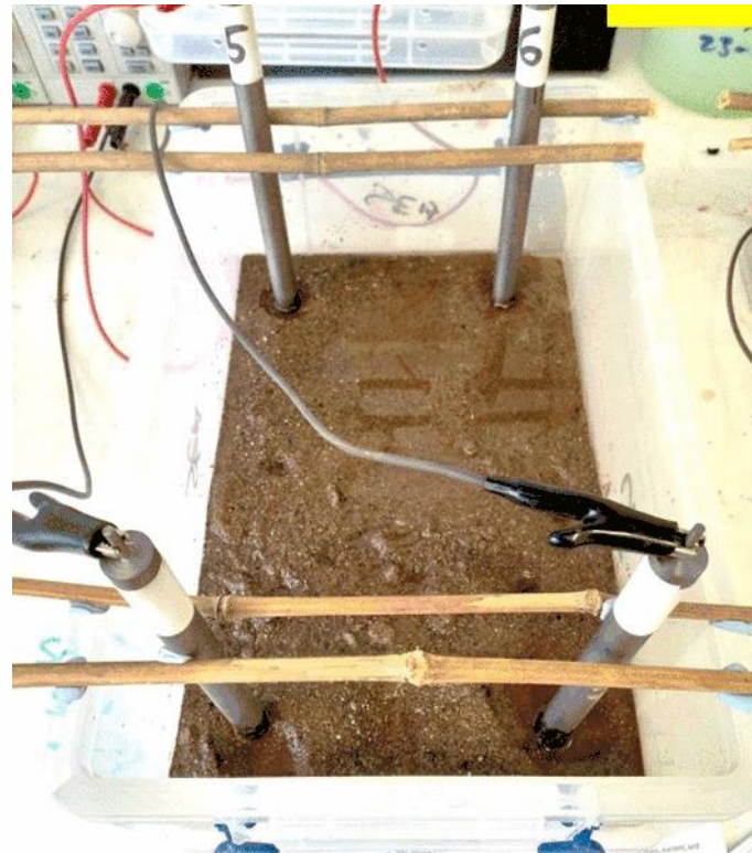
Sand with SW electrolyte (GIF starts at day 0)
