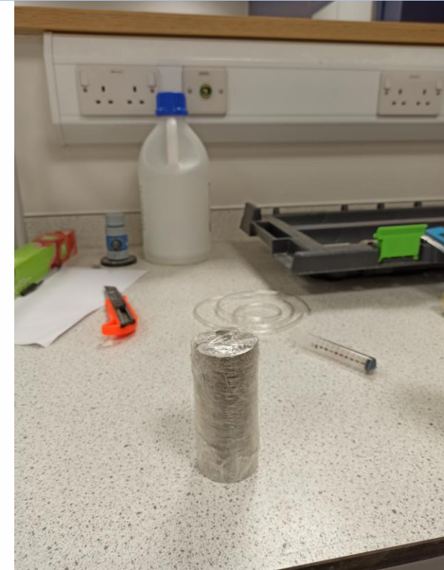
The half-cores wrapped together with membrane layers
