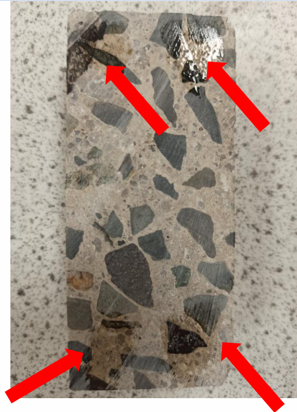
0.5mm diameter glass beads on the half- core's surface
