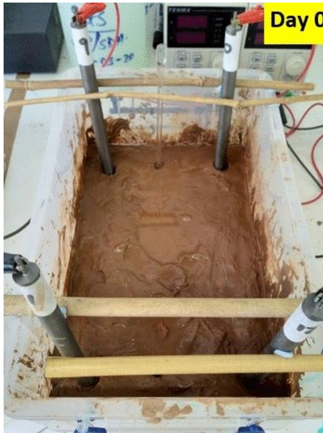
Clay with GW electrolyte
