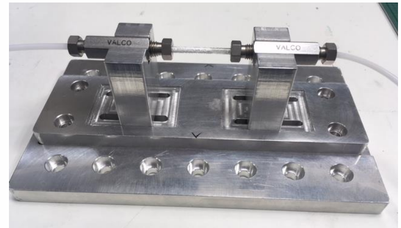
Figure 2 – the in-situ flow cell used for the exchange experiments
