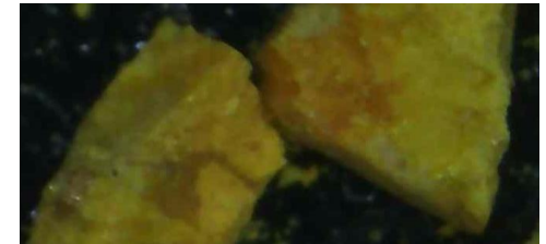
Becquerelite (?) \text{Ca}(\text{UO}_2)_6\text{O}_4(\text{OH})_6 \cdot 8(\text{H}_2\text{O})
